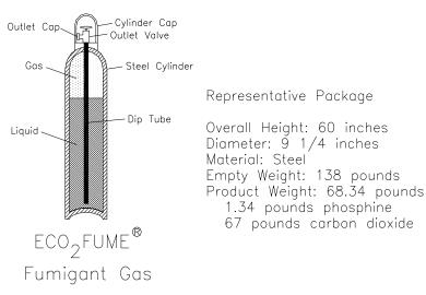
As liquid is withdrawn from the cylinder, some of the product vaporizes to fill the remaining space in the cylinder. Through this vaporization, the cylinder pressure is maintained.
